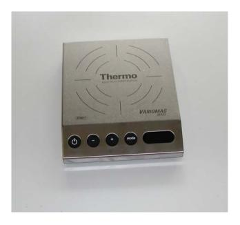
The Variomag Maxi direct-controlled magnetic stirrer is featured with pre-selectable power settings which optimize stirring efficiency for different liquid volumes and minimize heat output. Memory function stores the most recent settings, even when the device is unplugged for longer period of time. Stirring volume up to 5.000 ml and a far-reaching magnetic field makes the Variomag Maxi Direct suitable for highly viscous media.
